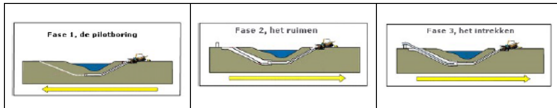
Figure 6: Phases of the HDD process
